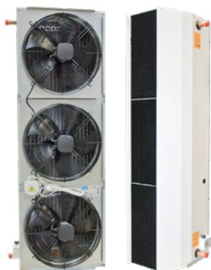
Robust construction with modular design, to be able to adjust the curtain to the size of the door. IP44 protection in all models except version with electric coil (IP20). Covers up to 12 m wide door, installing curtains on both sides. The equipment works without special controls. The controls add additional functions.
