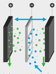
Particulate matter is ionized and becomes attached to oppositely charged collector cells and thereby removed from the outlet air flow.
